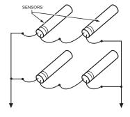
TO T775 CONNECTIONS (SENSOR A) OR (SENSOR B).  $$^{\rm M2}$$
