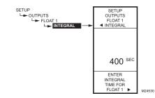
Fig. 64. Setup - Outputs - Floating Relay - Integral.
