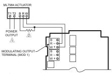
USE SEPARATE TRANSFORMER FOR T775R WHEN USING 24 VAC.
