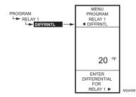
Fig. 29. Program - Differential or Throttling Range.
