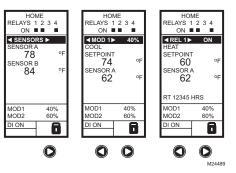
Fig. 23. LCD Display - Home Screen Displaying Sensors, Active Relays, and Mod Outputs.
