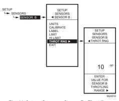
Fig. 44. Setup - Sensors - Sensor B - Throttling Range.
