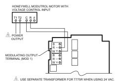
Fig. 16. Wiring for Modulating Actuator with Voltage Control Input.
