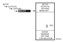
Fig. 56. Setup - Outputs - Options - Min Off Time.
