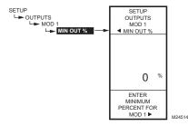
Fig. 48. Setup - Outputs - Mod Out - Minimum Output Percentage.
