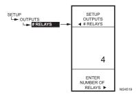
Fig. 53. Setup - Outputs - Number of Relays.
