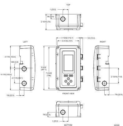
Fig. 1. T775A/B/M Dimensions in inches (mm).
