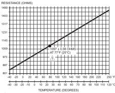
POSITIVE TEMPERATURE COEFFICIENT (PTC) OF 2.1 OHMS PER °F M243
