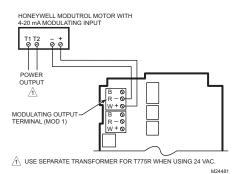
Fig. 14. Wiring for 4 to 20 mA Actuator.
