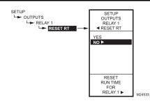
Fig. 67. Setup - Outputs - Relay - Reset Runtime.
