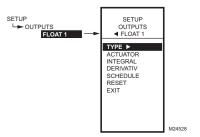
Fig. 62. Setup - Outputs - Floating Relay - Menu.
